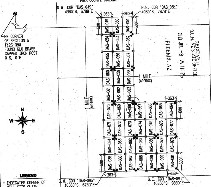
□ INDICATES CORNER OF MILL SITE CLAIM. SET 2"x2"x5' WOODEN POST (TYPICAL)
